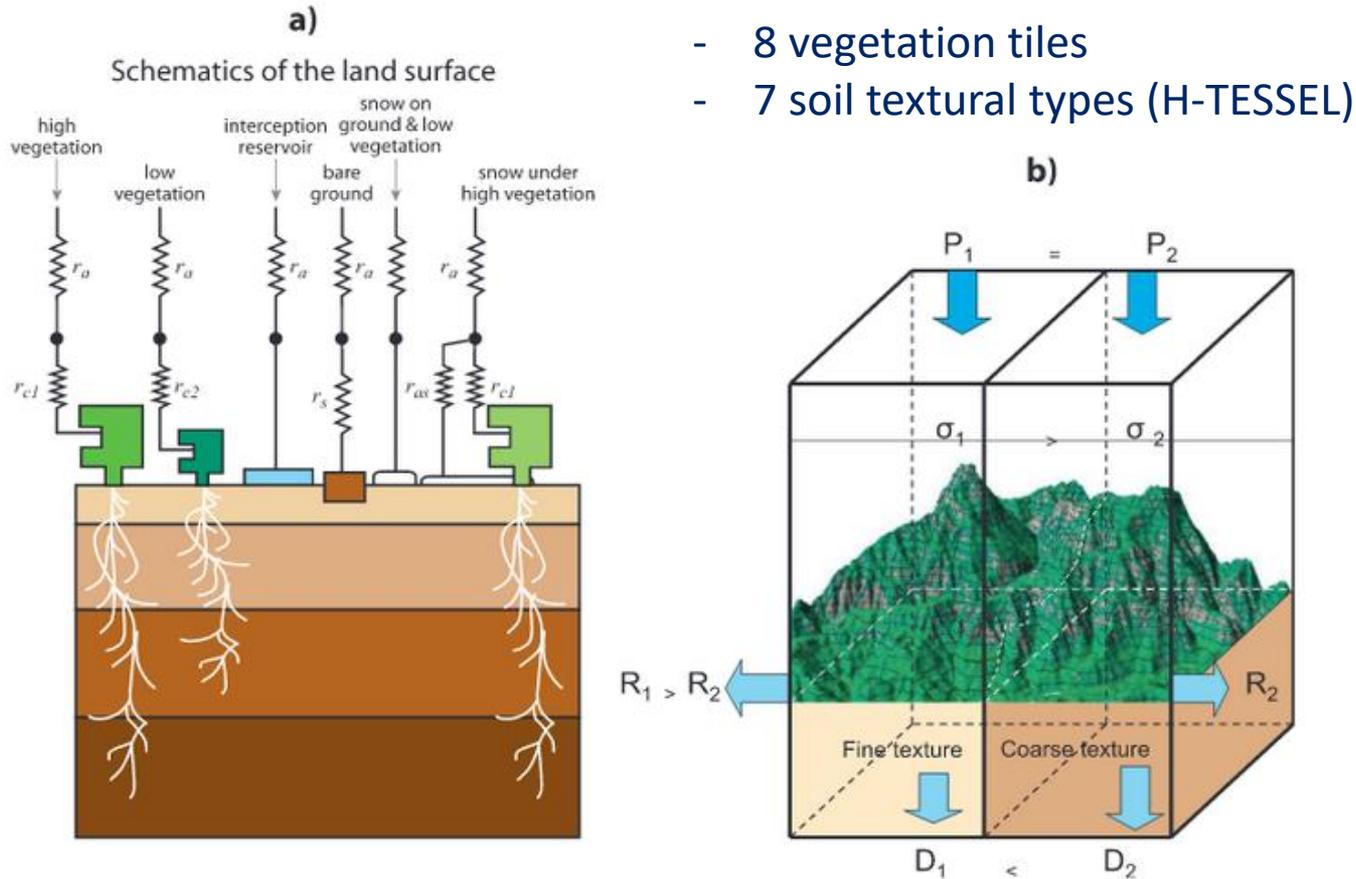
Figure 1: Schematic representation of the structure of (a) TESSEL land-surface scheme and (b) spatial structure added for H-TESEL. From Balsamo *et al* (2009).
